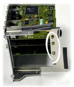
Image 2-7 The image is only intended to show where the plate must be mounted, (image does not reflect the reality since it shows a third layer (optional) which is not applicable when using a server).
